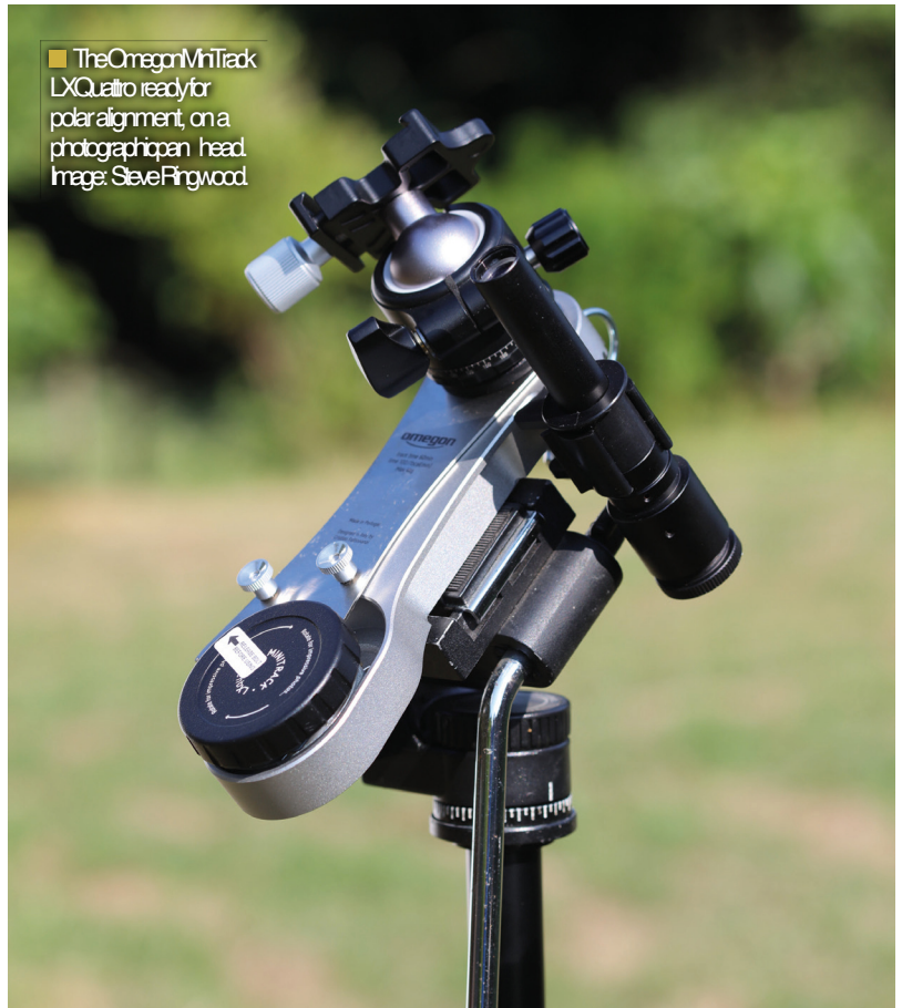
■ The MiniTrack fully kitted out, atop the deluxe wedge and fitted with Omegon's ball head and the reviewer's Canon 6D with a 100mm lens. Image: Steve Ringwood
